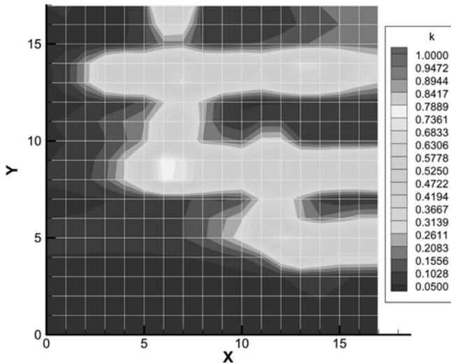
**Fig. 2.** The detected hydraulic conductivity field reflecting fracture pattern, based on the steady hydraulic tomography.
