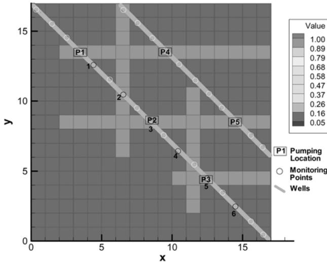
**Fig. 1.** The orthogonal fracture pattern and location of slanted pumping wells used in the numerical experiment. The hydraulic conductivity of the fracture (red) and that of the rock matrix (blue) are 1m/s and 0.05 m/s, respectively.
