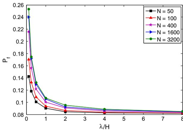
Fig. 4. Effect of the number of potential slip surfaces ( $N$ ) on  $p_f$  at different values of correlation scale based on Example 1.
