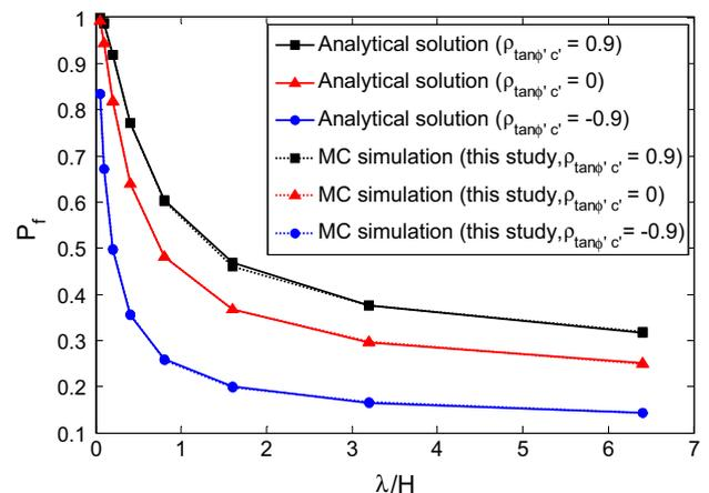
Fig. 6. Comparison of  $p_f$  by analytical approach and MC simulation (this study) for Example 3 with normal distributed properties showing the influence of correlation scale and correlation coefficient  $\rho_{\tan \phi' c'}$ .
