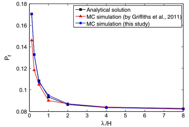
Fig. 2. Comparison of  $p_f$  by analytical approach and MC simulation (by Griffiths et al. [11] and by this study) for Example 1 showing the influence of correlation scale.
