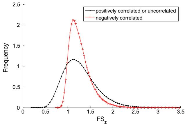
Fig. 8. Illustration for probability density distribution of  $FS_z$  when  $FS_z$  is the sum of two log-normal distributed random variables.
