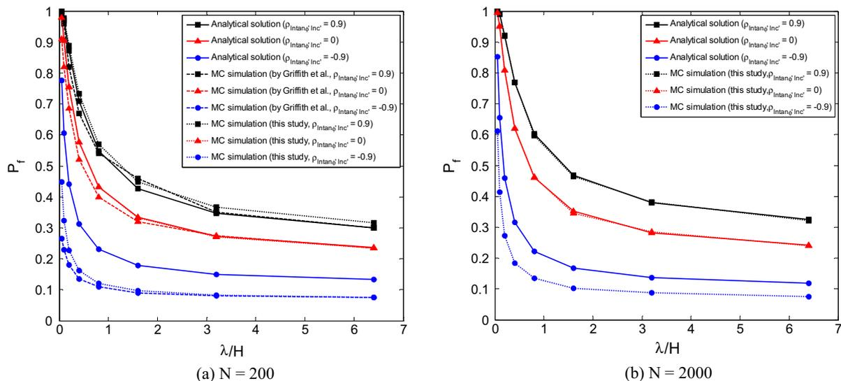
Fig. 7. Comparison of  $p_f$  by analytical approach based on first-order approximation and MC simulation (by Griffiths et al. [11] and by this study) for Example 3 with log-normal distributed properties showing the influence of correlation scale and cross-correlation coefficient  $\rho_{\tan \phi' c'}$ .
