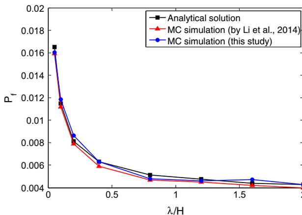
Fig. 5. Comparison of  $p_f$  by analytical approach and MC simulation (by Li et al. [12] and by this study) for Example 2, showing the influence of correlation scale.
